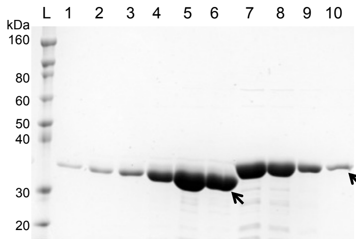
Figure 6-18. SDS-PAGE analysis of fractions from peaks eluted at 0% (v/v) (\text{NH}_4)_2\text{SO}_4 at a large scale HIC purification of modular VP1 capsomeres. (L) Pre-stained protein marker, (1-6) TEVP-H190, and (7-10) TEVP-GCN4-H190-GCN4. Black arrows refer to VP1.
