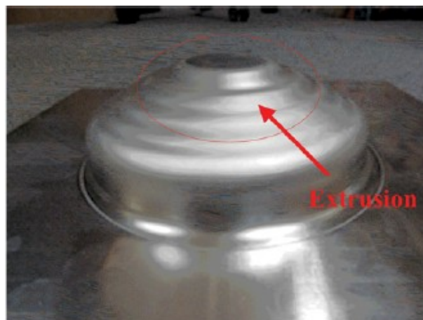
Fig.2.8. Material extrusion phenomenon in multi-pass SPIF ( Paper G ).
