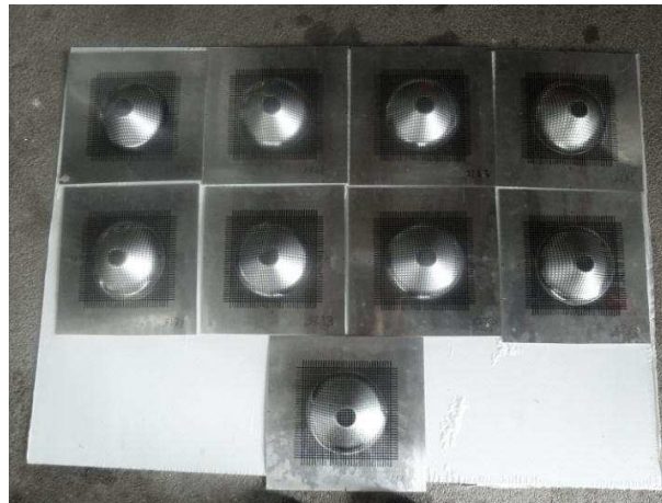
Fig.3. The nine formed truncated cones according to Taguchi design.
