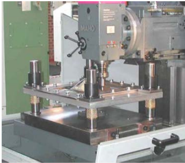
(a) Conventional milling machine upgraded and used for ISF.
