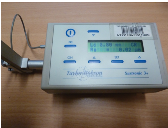
FIGURE 9.—Taylor-Hobson Surtronic 3+ Profilometer.
