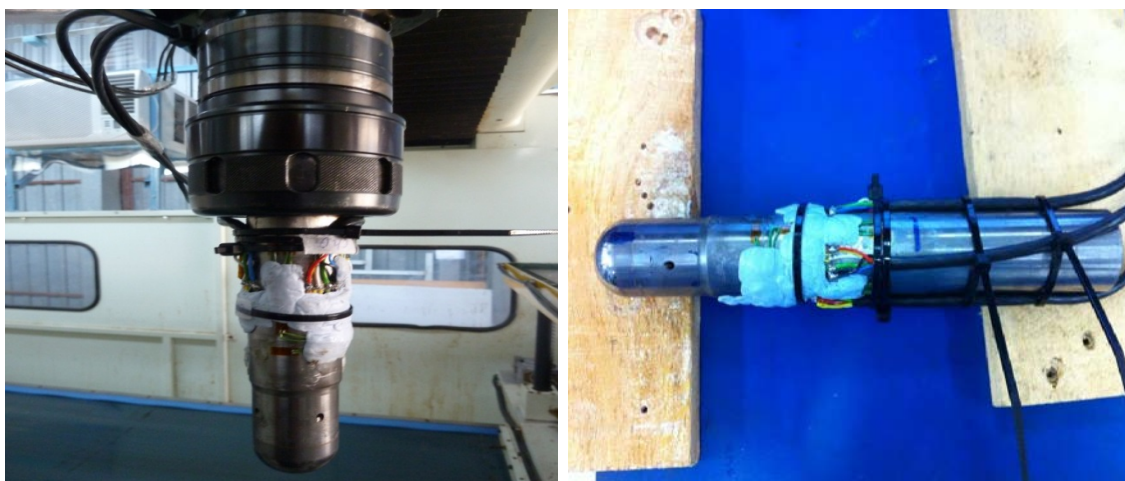
Fig.3.10. Simplified load cell for the force measurement.
