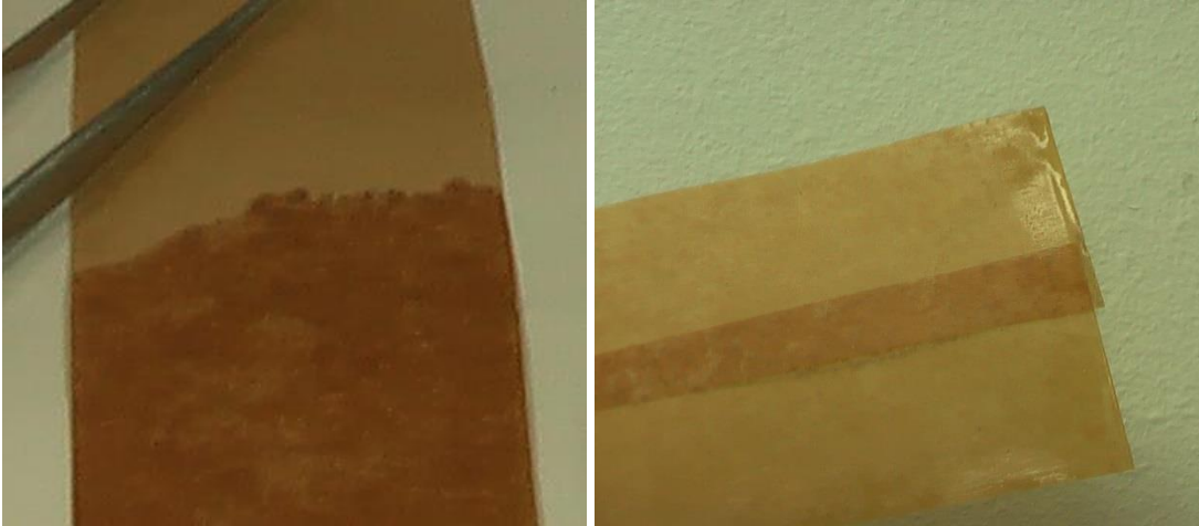
Figure 13: Varnish like substance on paper (left), gel on edge of paper (right)
