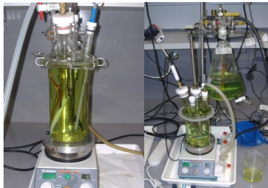
Figure 2: Vessel used to age vegetable oil. Left – Oxygen was bubbled through oil. Right – A conical flask conservator was attached to the vessel, and the headspace within the conical flask was filled with dry argon gas to minimise ingress of oxygen.
