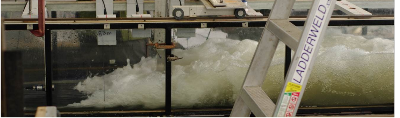
Figure 1 – Experimental hydraulic jump - Flow conditions: Q = 0.0399 \text{ m}^3/\text{s} , d_1 = 0.020 \text{ m} , x_1 = 0.83 \text{ m} , Fr_1 = 8.5 , Re = 7.9 \times 10^4 - Flow direction from left to right
