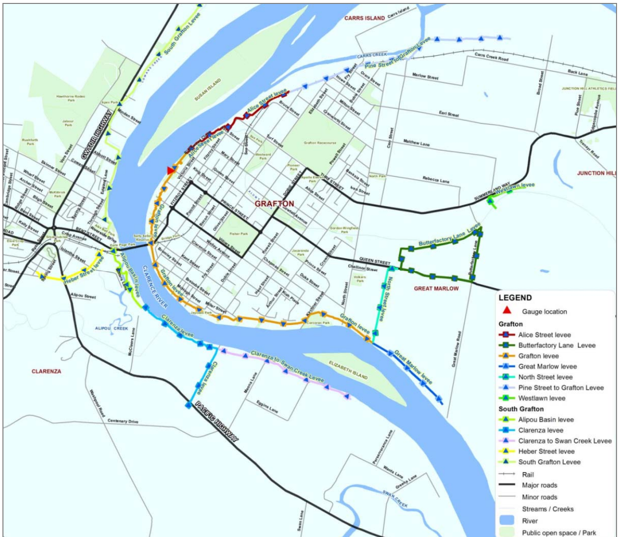
Figure 1 - Grafton and South Grafton Levee system
