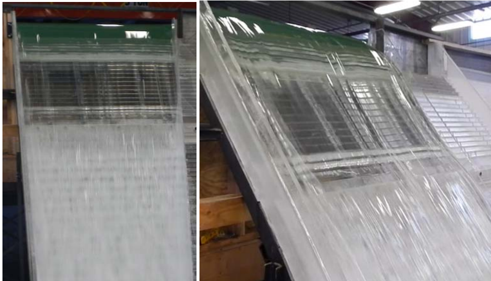
Figure 6 – Chute flow at PMF discharge
