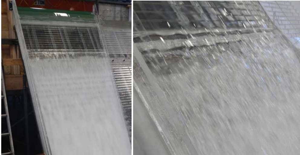
Figure 5 – Chute flow conditions at the AEP 1 in 10,000 discharge
