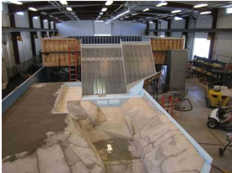
Figure 1 – General view of the two-spillway concept model
