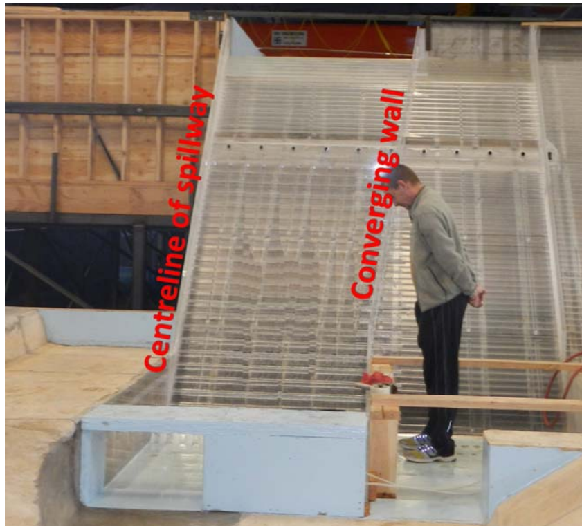
Figure 2 – Convergent chute half model
