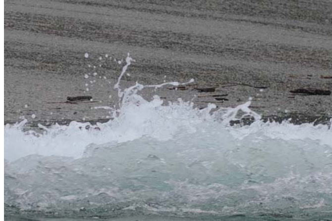
(C) Hydraulic jump roller and details of upper spray region along Katashima River at Oigami township (Japan) on 7 October 2012 (shutter speed: 1/8,000 s)
