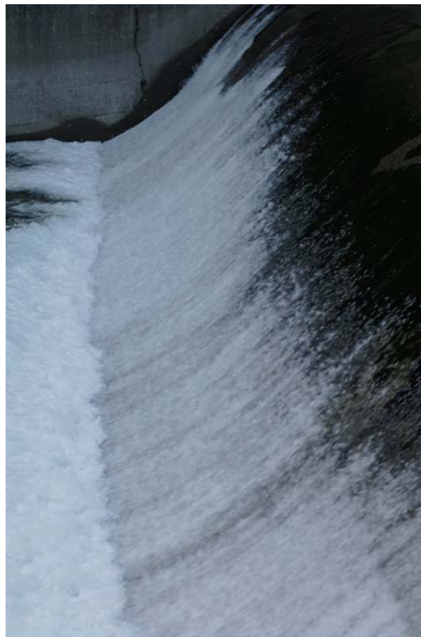
(C) Hydraulic jump at a weir toe on Ogika River, upstream of Ikari dam, Tochigi Prefecture (Japan) on 8 October 2012 - q \sim 0.1 \text{ m}^2/\text{s} , Re \sim 1 \times 10^5
