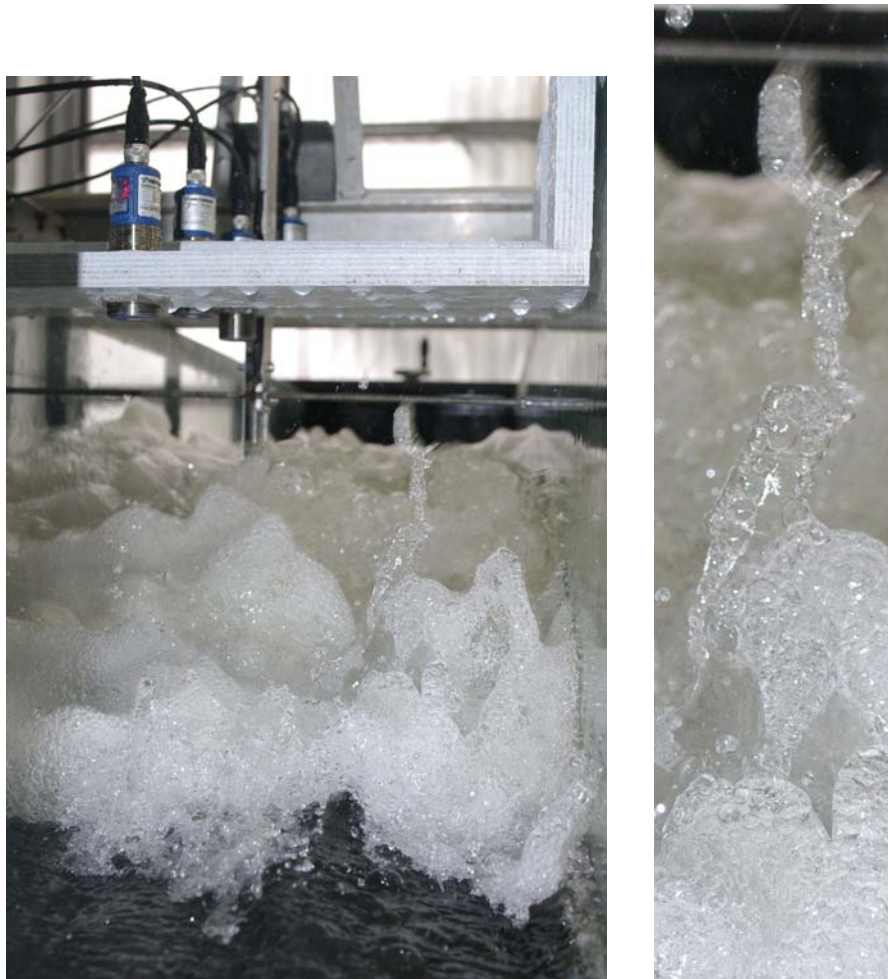
(C) Looking downstream, viewed from upstream of jump toe - Inset: details of air-water projection Fig. F-2 - Hydraulic jump experiment - Flow conditions: Q = 0.0399 \text{ m}^3/\text{s} , d_1 = 0.020 \text{ m} , x_1 = 0.83 \text{ m} , Fr_1 = 8.5 , Re = 7.9 \times 10^4 - Shutter speed: 1/80 \text{ s}
