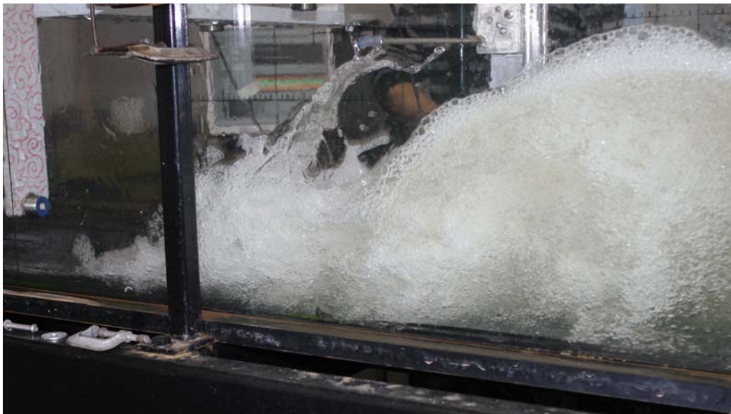
(B) Three-quarter view highlighting large air-water projection, flow direction from left to right
