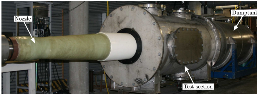
(b) Nozzle, test-section and dump-tank [17].
