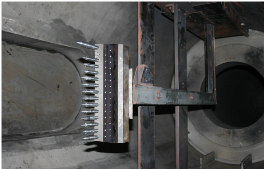
(c) Pitot probes in test section [17].
