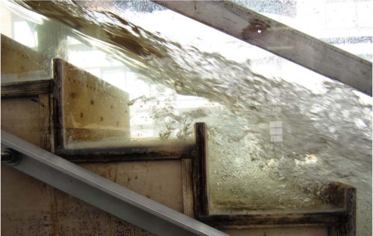
Fig. 3. Skimming flow regime on the porous pooled stepped spillways
