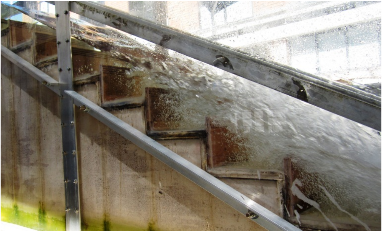
Fig. 3. Skimming flow regime on the porous pooled stepped spillways
