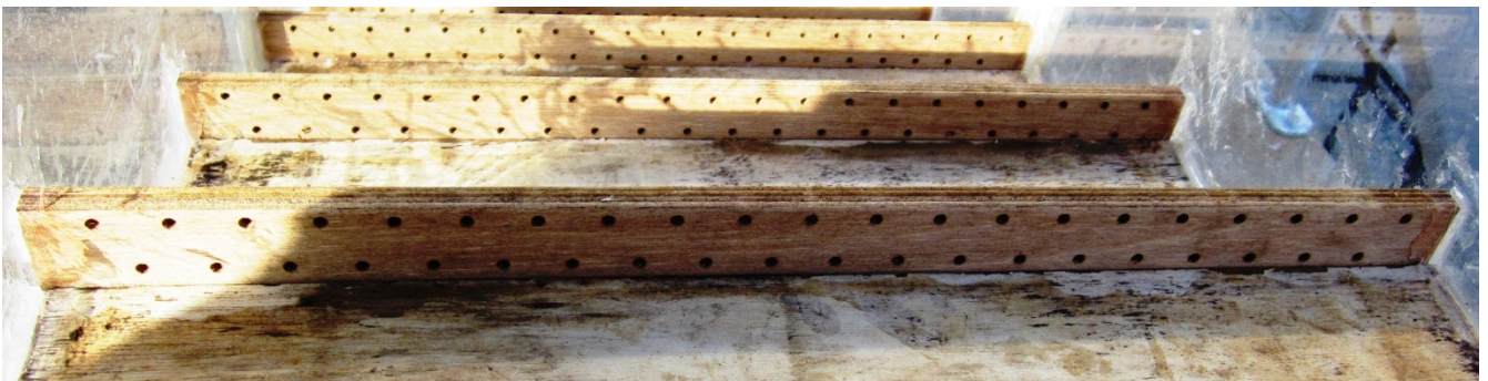
Fig. 1. Stepped spillway configurations with flat, pooled and porous pooled steps ( \theta = 26.6^\circ )
