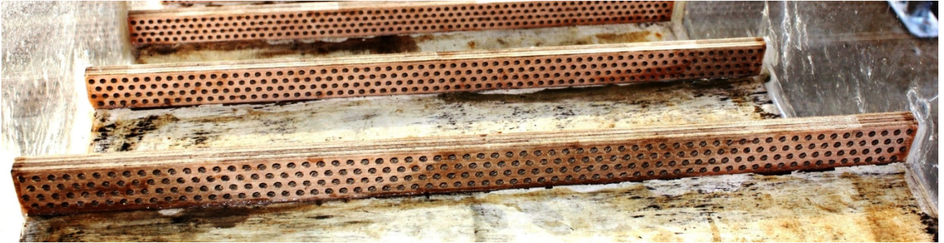
Fig. 1. Stepped spillway configurations with flat, pooled and porous pooled steps ( \theta = 26.6^\circ )
