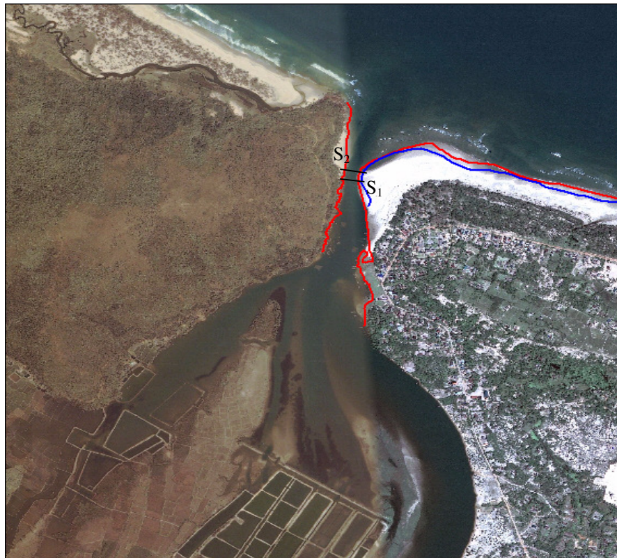
Figure 5.3: Canh Duong inlet, Hue, Vietnam, shorelines measured in 27 February 2010 (—) with two velocity transects ( S_1 , S_2 ) and shorelines measured in 13 February 2011 (—) plotted on Google Earth image 22 February 2009.
