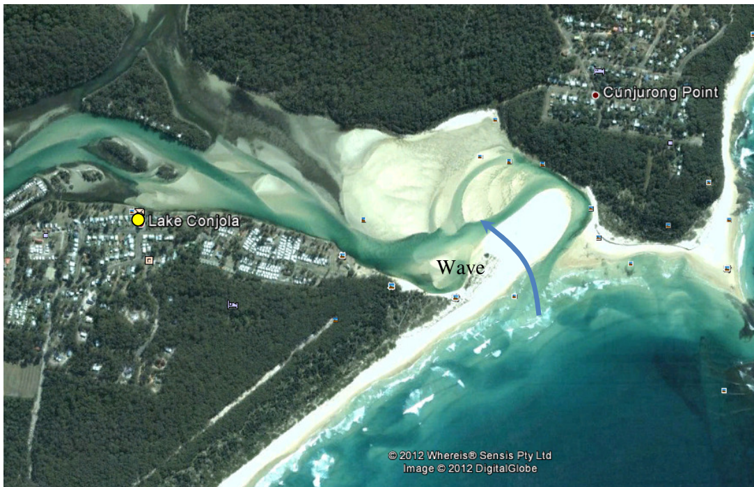
Figure 2.9: Lake Conjola, NSW, Australia (Google Earth image) where a significant flood event driven by wave overwash occurred in April 2006. The vegetation pattern gives an indication as to which part of the spit is regularly overtopped by waves.
