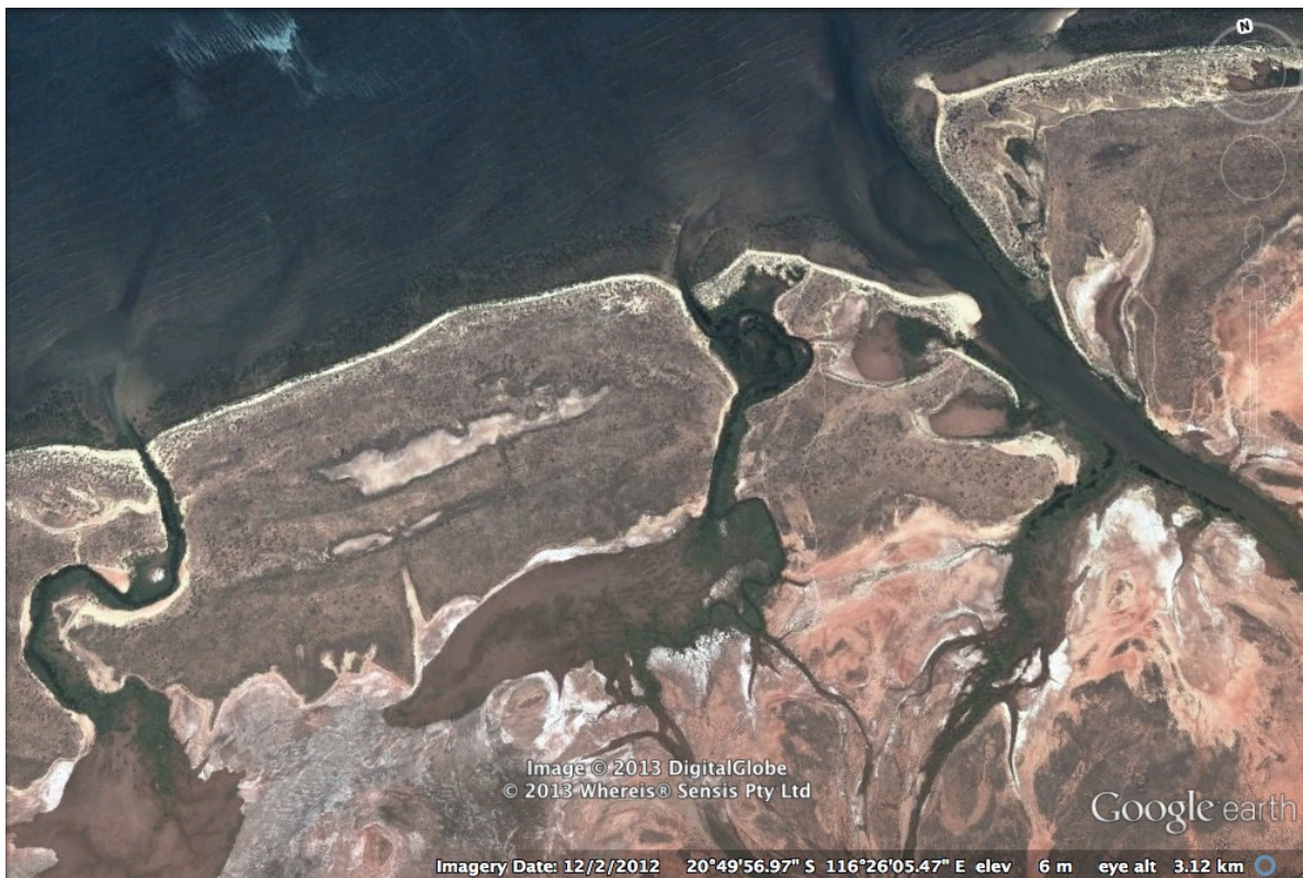
Figure 1.9: Three neighbouring inlets at 20°49’S 116°26’E in Western, Australia. In this area the spring tidal amplitude is around 2.2 m and the tides are predominantly semi-diurnal. The mean significant wave height is of the order 0.7 m, Baldock et al (2006).
