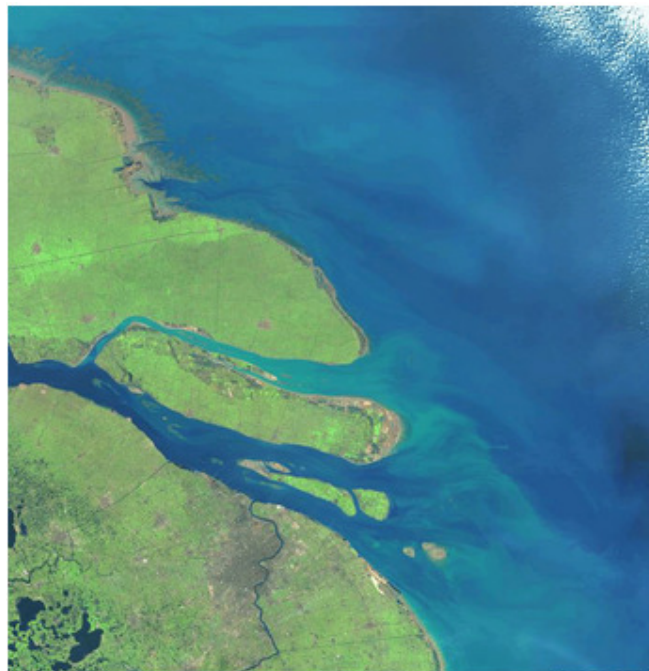
Figure 1.8: Yangtze-Kiang, China: An example for highly tide-dominated coast with low wave energy and a large \overline{Q_{tide}} , tidal amplitude = 3.8 m (from World delta data base, 2004).
