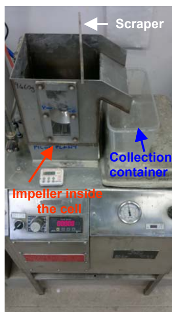
Figure 6-19 The standard JKMRC flotation cell
