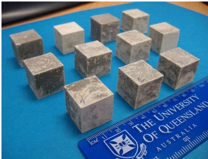
Figure 4-4 Cubes made of Quartz sand, PMMA and pyrite grains
