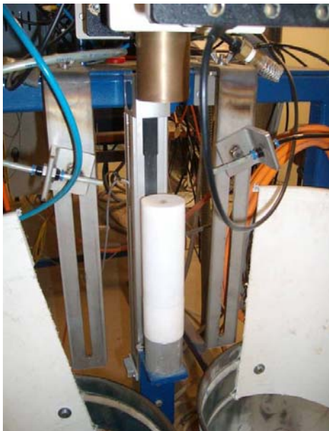
Figure App. A-5 Particle holder made out Teflon ®
