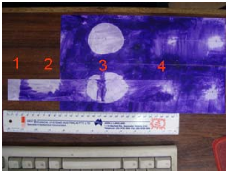
Figure 3-30 Thermal paper patterns from both exposures
