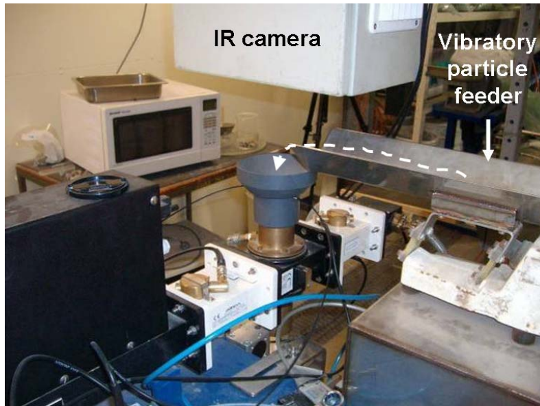
Figure 4-34 Feeding and inspection part of the travelling wave applicator
