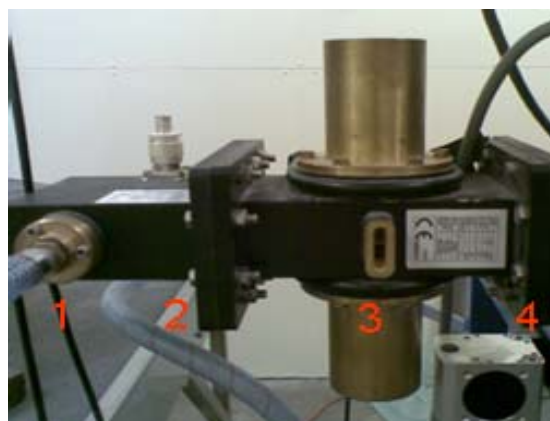
Figure 3-29 TWA applicator with dummy water load
