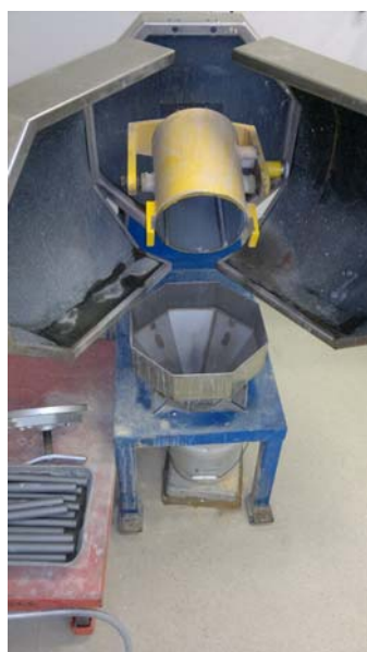
Figure 6-18 Rod mill used to grind samples for 10 and 15 minutes
