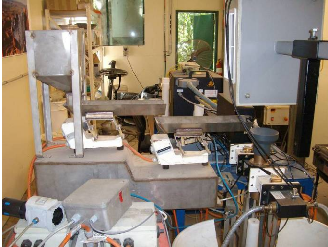
Figure App. A-8 Two vibratory feeders with different speeds used to supply continuous flow of particles one by one
