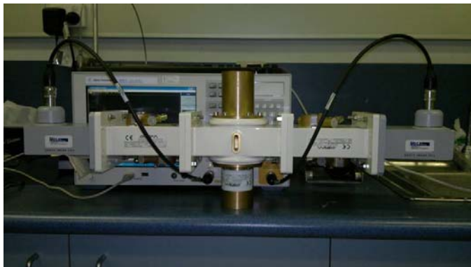
Figure 4-25 The resonant cavity from outside
