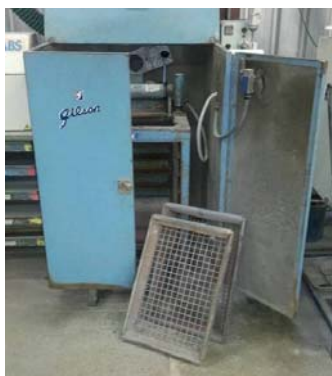
Figure 5-2 The Gilson Testing Screen used to screen material into fractions.
