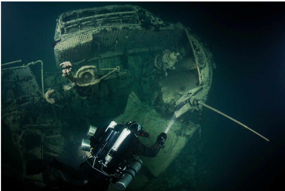
The badly damaged conning tower of German World War II submarine U-479. She was sunk by a mine in the late autumn of 1944 and rests on the seabed at 95 metres. (Picture: Jouni Polkko, courtesy of badewanne.fi, 2015.)
