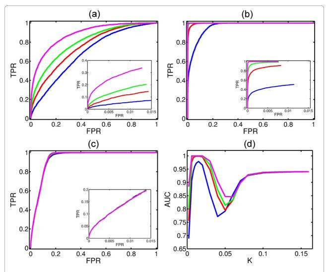
**Figure 5 Reconstruction of Underlying Struture from WNS.** ROC curves to depict the reconstruction of physical connectivity with one (blue), three (red), five (green) and ten (magenta) initial configuration(s) as the coupling strength K = 0.002 (a), K = 0.010 (b) and K = 0.100 (c). The insets in (a-c) are the corresponding ROC curves up to the first 2000 predicted links. Plotting AUC versus K helps to find the optimal regime of coupling strength for reconstruction of physical connectivity (d).
