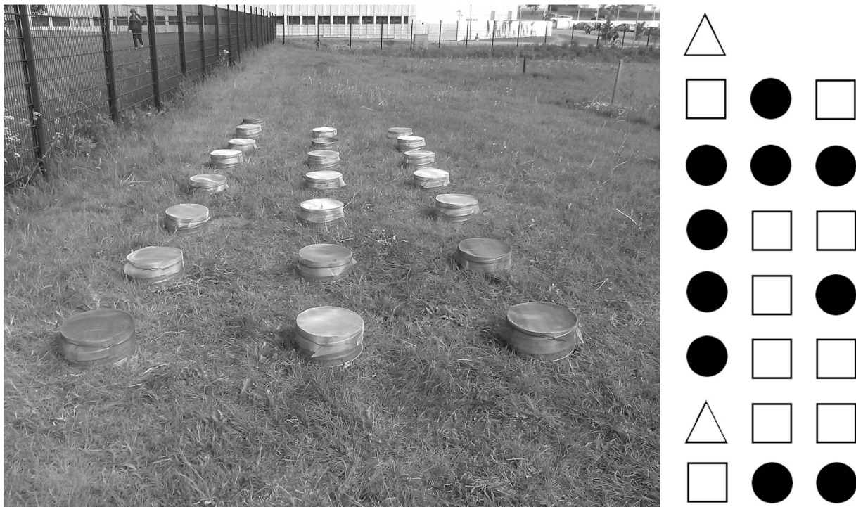
Figure 1. Experimental design used in measuring gas fluxes. (A) Twenty-two mesocosms were placed in an agricultural field, separated by distances of 70 cm. (B) These mesocosms were randomly assigned to three different treatments: 1) dung with dung beetles (open squares; n = 10 ); 2) dung without dung beetles (filled circles; n = 10 ), and 3) chambers containing neither dung nor beetles (open triangles; n = 2 ). doi:10.1371/journal.pone.0071454.g001
