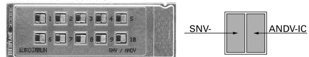
Figure 1. Immunofluorescence microscope slides for the multiparametric detection of hantavirus-specific antibodies. A microscope slide has ten reaction fields, each of which contains a biochip mosaic, allowing ten samples or sample dilutions to be incubated simultaneously with the same range of substrates. Due to identical incubation protocols, IgG and IgM testing can be performed on different reactions fields of the same slide using the respective secondary antibody conjugate. Hantavirus Mosaic 1 comprises mosaics of six biochips coated with Hantaan virus (HTNV)-, Puumala virus (PUUV)-, Seoul virus (SEOV)-, Sin Nombre virus (SNV)-, Dobrava virus (DOBV)- and Saaremaa virus (SAAV)-infected cells (-IC). Hantavirus Mosaic 3 consists of mosaics of two biochips coated with Sin Nombre virus (SNV)- and Andes virus (ANDV)-IC. doi:10.1371/journal.pntd.0002157.g001
