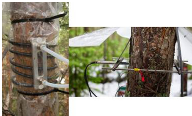
Figure 2. The stem enclosure around a Scots pine stem at a height of 12 m (left) and a linear variable displacement transducer to measure stem radius changes (right).
