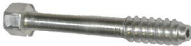
Figure 2: Aluminium screw employed. The screw was custom manufactured from high grade aluminium; the geometry was based on a commercially available partially threaded cancellous lag screw from Smith and Nephew (Catalog No. 7111-9106, Smith and Nephew, London UK).
