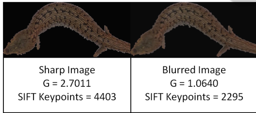
Figure 4: A side by side comparison of a sharp and blurred image from the same sequence with the resulting total high frequency energy and SIFT keypoints.
