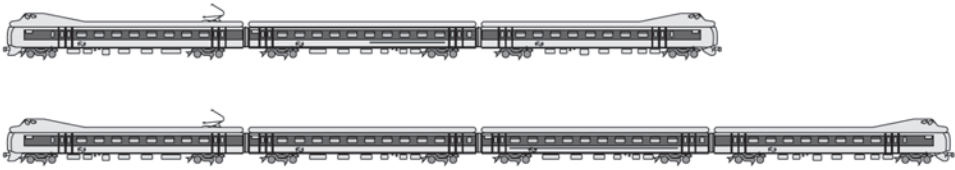
Figure 2.9. This figure illustrates two single-deck rolling-stock units with three and four carriages, respectively
