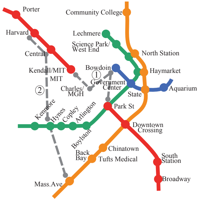
Figure 4.6: MBTA core network with shuttle lines operated in base case C_{\text{shut}} solution.
