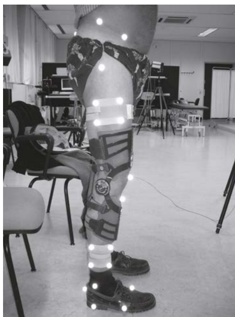
Fig. 3. Lateral view of the right knee showing MOS Genu ® knee brace with fixated markers.
