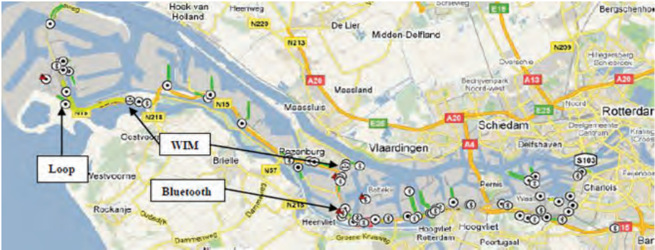
Figure 1.1: The locations of Bluetooth devices, WiM systems and loop detectors around the A15 motorway. (Source: Reportis.com)
