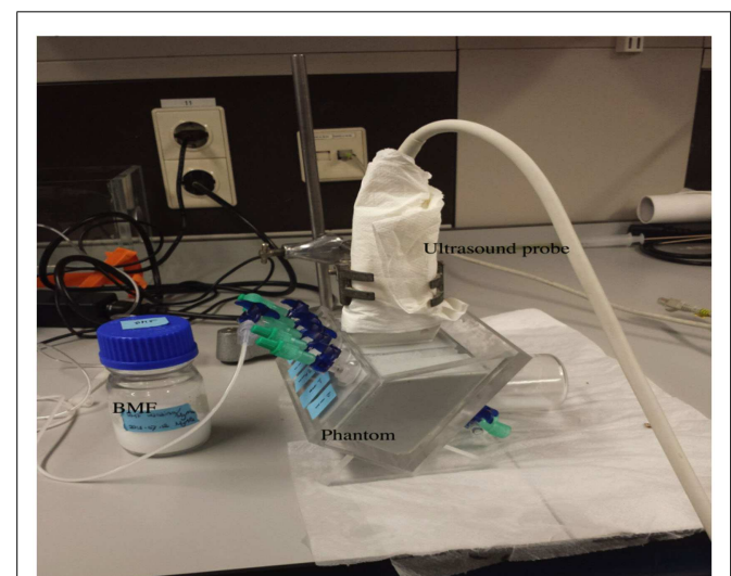
FIGURE 1 | The test setting. Flow phantom with a fixed ultrasound probe. BMF, blood-mimicking fluid.
