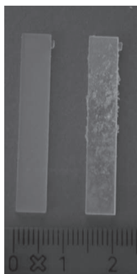
Fig. 5 PP plates with hydrophilic poly(PEGMA) grafted in the absence (left) and in the presence (right) of a sacrificial initiator.
