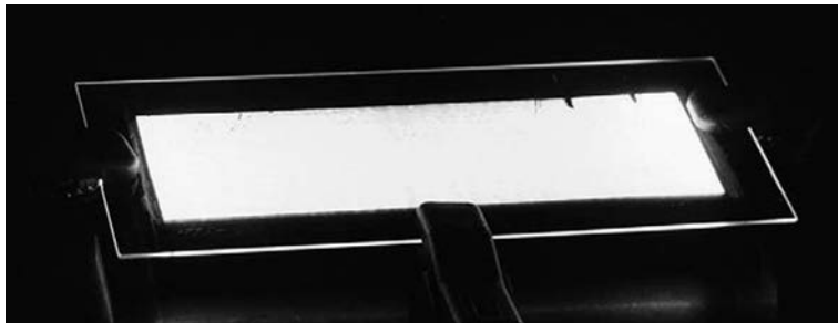
Figure 7.9 Gravure-printed large-area OLED (active area 30 cm 2 ) with two printed organic layers (PEDOT and a blue-emitting layer – colour does not show). Reproduced from Kopola et al. (2009) with the permission from Elsevier.
