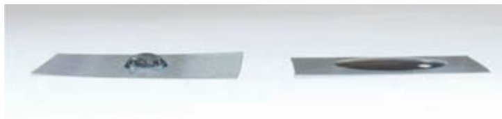
Fig 5.13 – contact angle measurements reprinted with permission from reference 5.
