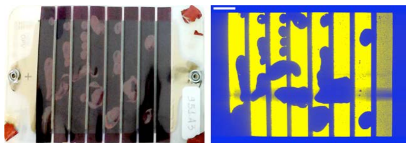
Fig. 5. (Left) front picture of a degraded AgNW module with Ag grid in the back after ISOS-L-3. (Right) LBIC of the same module where the light yellow areas correspond to photovoltaic function and the blue areas to non-active or destroyed areas.
