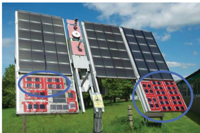
Figure 5. Carbon freeOPV modules mounted outside on a sun-tracking platform during ISOS-O-1 testing (the modules circled in blue are fixed in groups with red tape).
