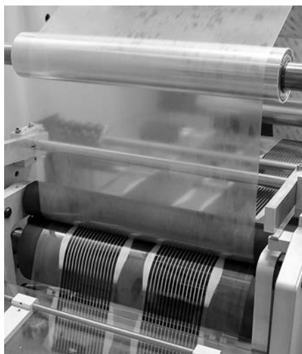
Figure 7.21 Hot lamination of organic solar cells modules.
