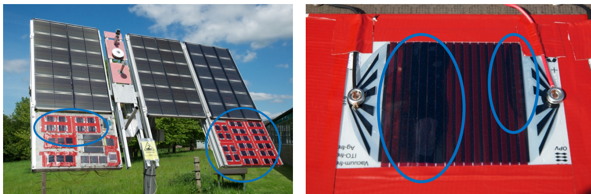
Fig 5.12 – (left) the freeOPV mounted on the sun tracking platform are circled in blue. (right) picture of a freeOPV module with water ingress (blue circle). Reprint with permission from 5.
