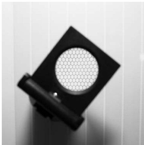
Figure 7.11 Example of a R2R ink-jet-printed silver grid.
