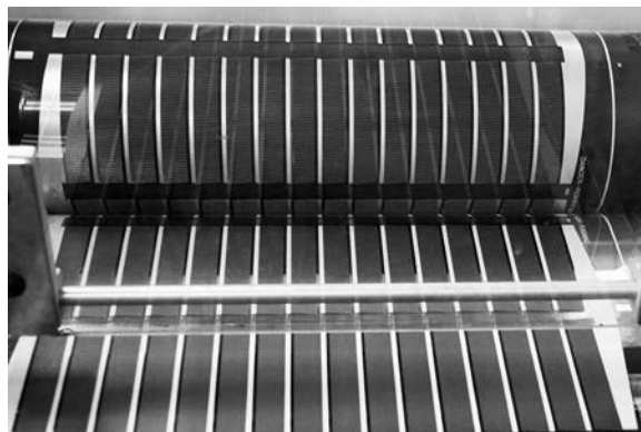
Figure 7.6 The printing cylinder with the relief carrying the ink (in this case a silver paste) during printing. The final printed pattern on the web can be observed in the bottom part of the picture.
