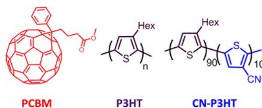
Fig. 1 Chemical structures of PCBM, P3HT, and CN-P3HT.
