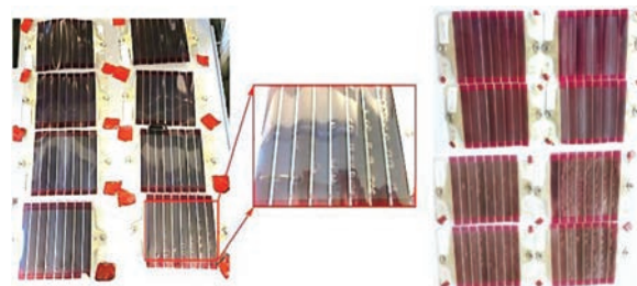
Fig. 7 Samples under ISOS-L-3 test with AgNW front electrode. Left: Samples after 2 weeks. Centre: Detail of the sample at the right bottom corner of the picture in the left. Right: Samples after finishing the test. Four samples on top are with PEDOT:PSS back electrode (no bubbles formed) and the four samples in the bottom with Ag-grid back electrode (extensive bubble formation).
