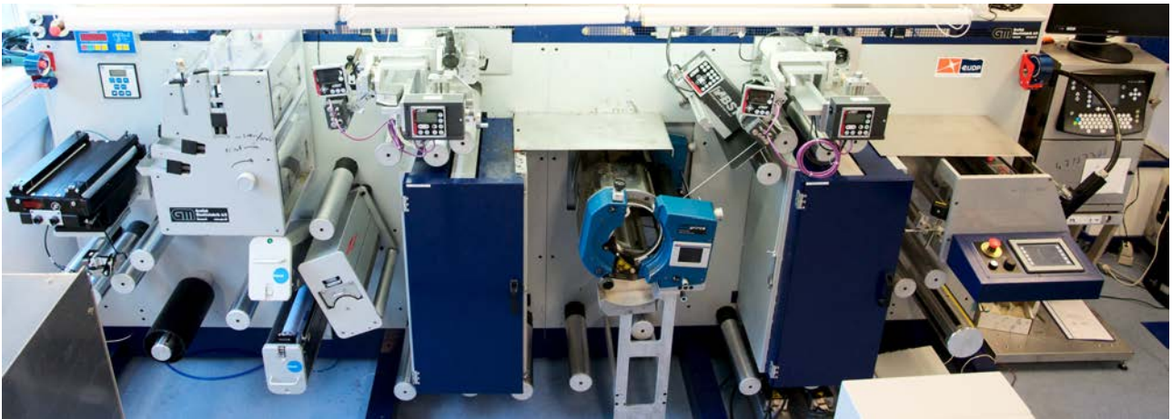
Fig 2.8 – Photograph of the R2R machine used for coating and printing of large scale OPV modules.
