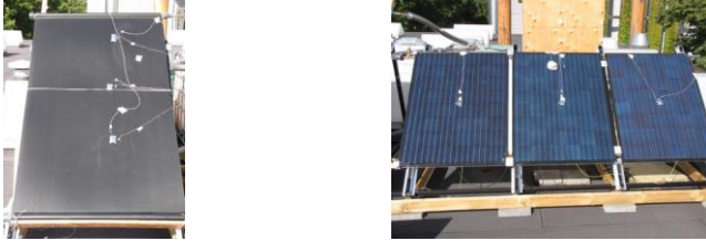
Figure 1. The studied unglazed solar collector (left), and the three PV/T panels (right). A schematic drawing of the experimental setup can be found in [4].
