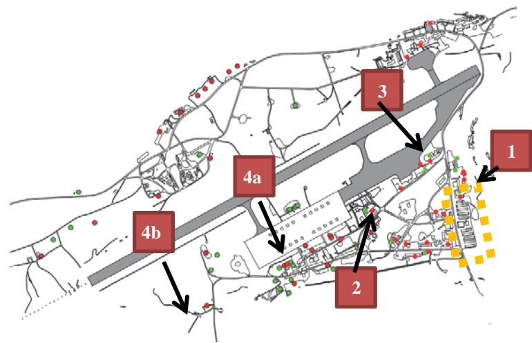
Figure 1. Red dots are potentially active (present) point sources and green dots are former or closed locations of dumps. Numbers 1-4b are observed and confirmed pollution sites.
