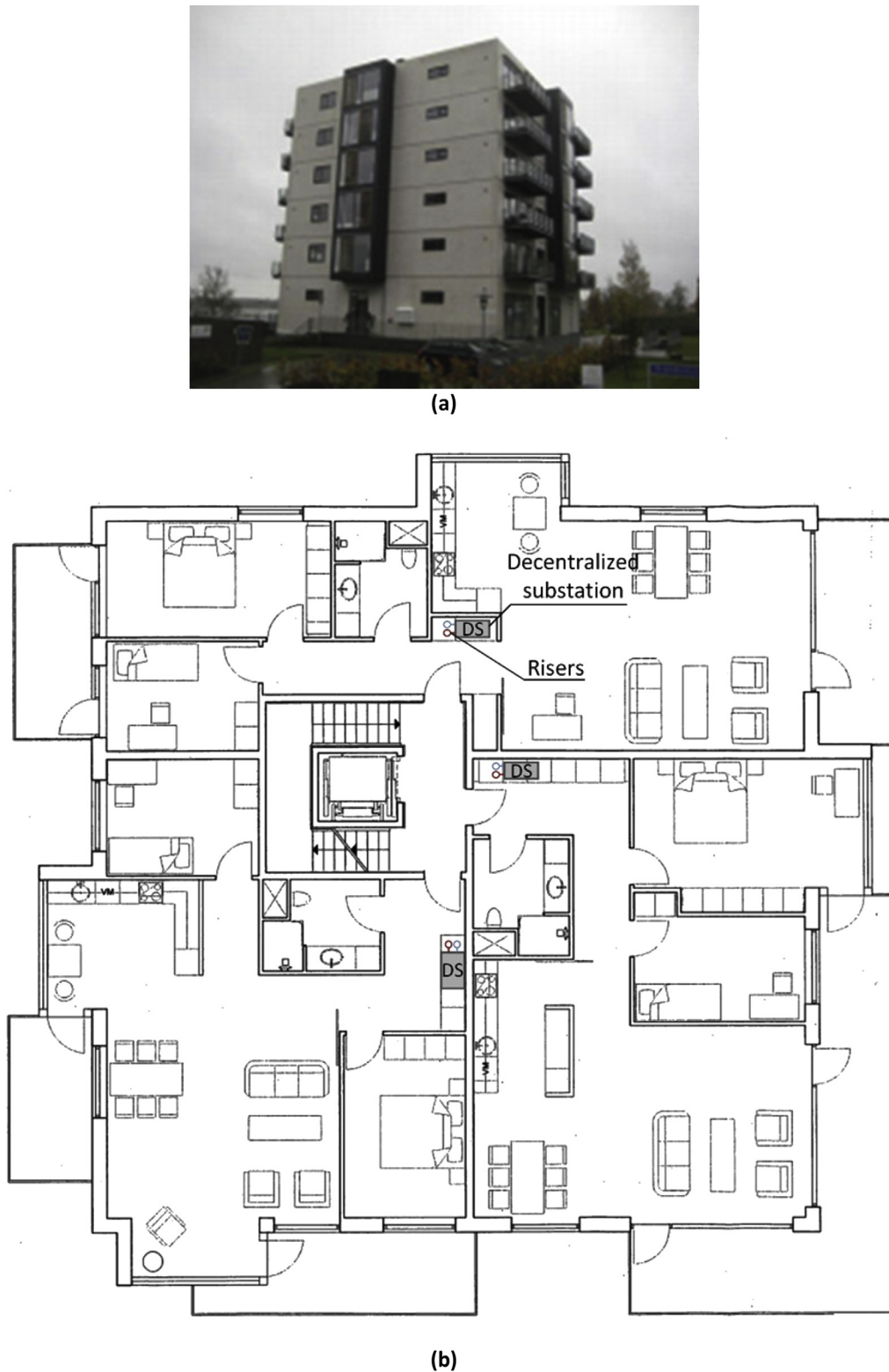
Fig. 1. The reference building (a) and the floor layout (b) of the residential storeys.
