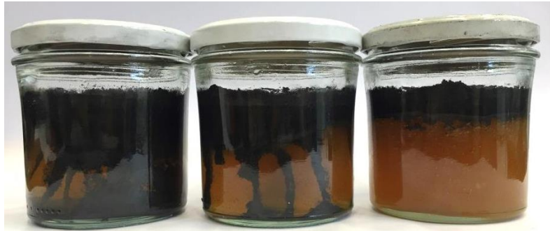
Figure 6. SAT samples with 0.25%, 0.5% and 1% Xanthan rubber with graphite powder on top after 14 days at 90 °C.
