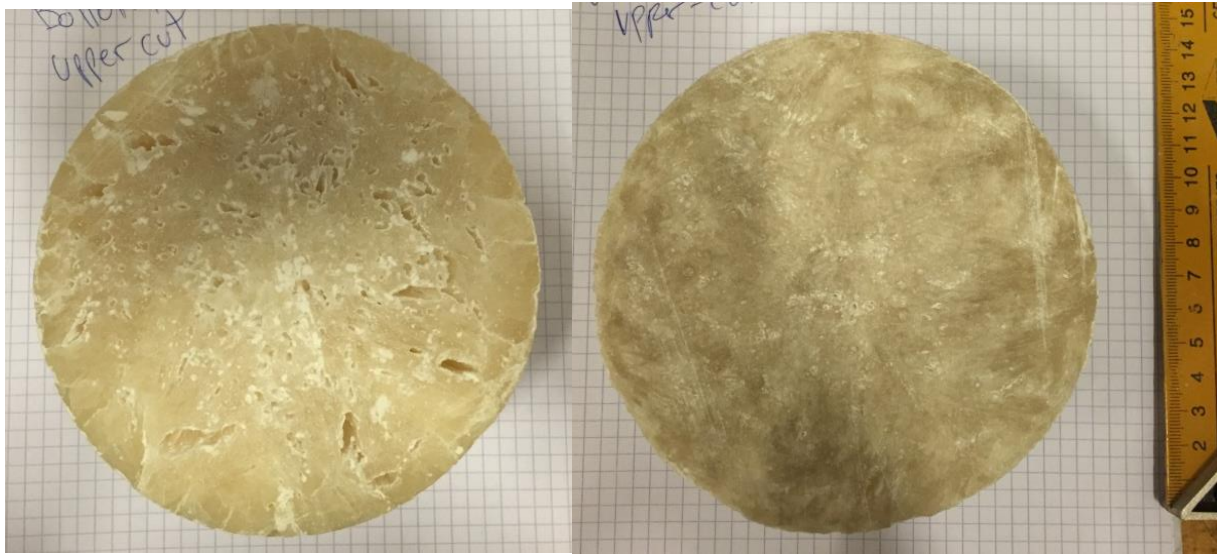
Figure 11. (a) SAT with 0.5% Xanthan rubber solidified without supercooling. (b) SAT with 0.5% Xanthan rubber solidified from supercooled state.
