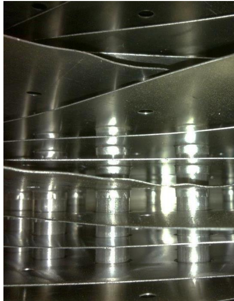
Figure 21. Internal heat exchanger of stainless steel pipes and aluminum fins.
