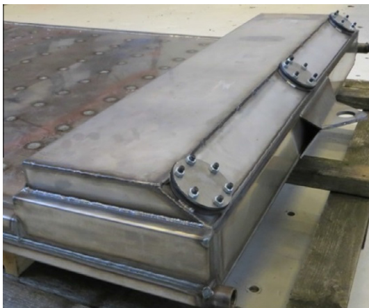
Fig. 4. Expansion volume with filling necks, rubber gaskets and lids.
