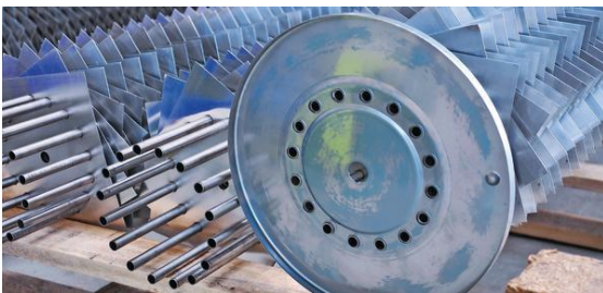
Figure 2. Internal heat exchanger [39].
