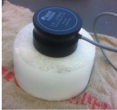
Figure 9. Applied Precision surface probe for measuring thermal conductivity on SAT sample.
