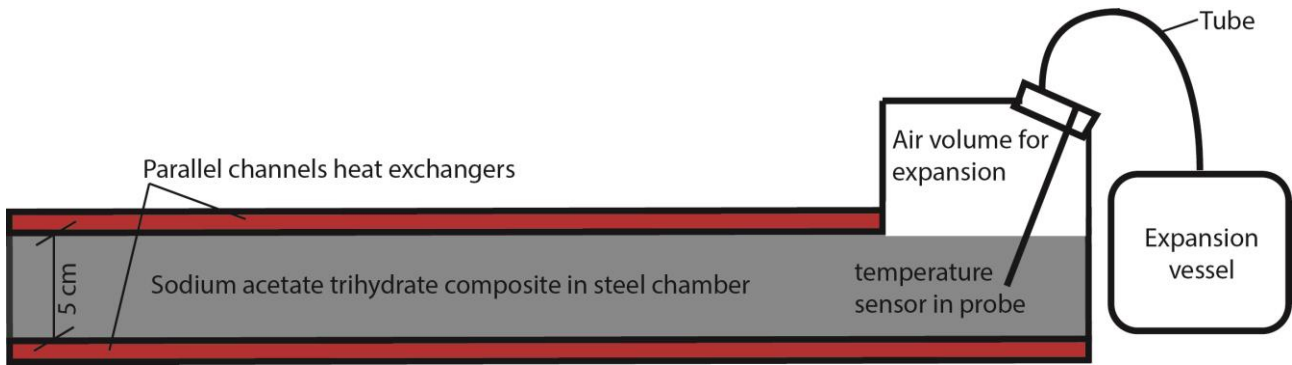
Figure 19. Principal diagram of flat heat storage unit with expansion.
