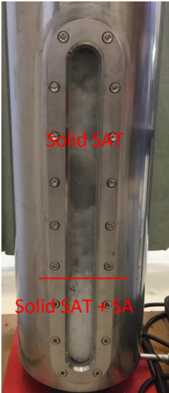
Figure 14. Bottom inspection window of unit with SATH20.
