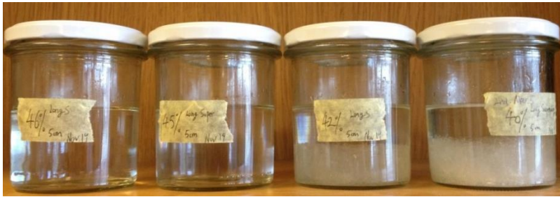
Fig. 4. The 40%, 42%, 45% and 46% salt water mixtures from right to left after 100 days supercooling
