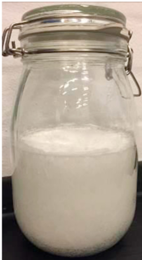
Fig. 2. 1.3 kg PCM composite based on SAT in glass jar.
