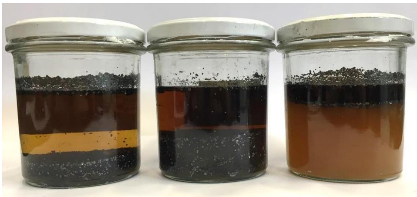
Figure 7. SAT samples with 1%, 2.5% and 5% CMC with graphite flakes on top after 14 days at 90 °C.
