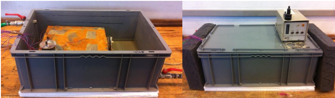
Figure 13. (a) Steel unit placed the thermostatic bath. (b) Closed thermostatic bath with controller.
