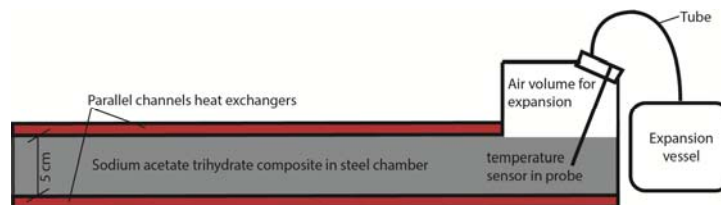
Fig. 2. Schematic module design with expansion vessel.
