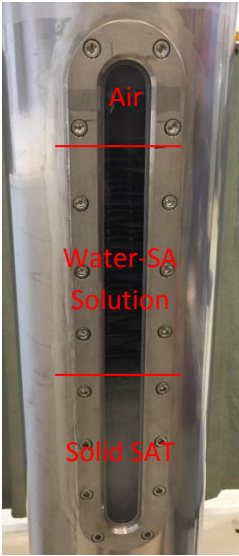
Figure 13. Top inspection window of unit with SATH20.
