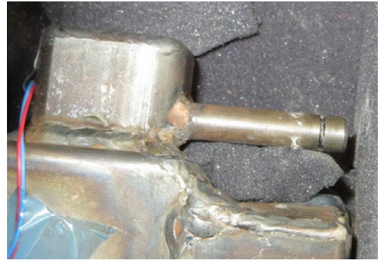
Fig. 5. CO 2 chamber for activating solidification of supercooled PCM mixture by cooling.
