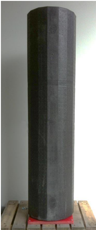
Figure 20. Cylindrical heat storage unit with insulation.
