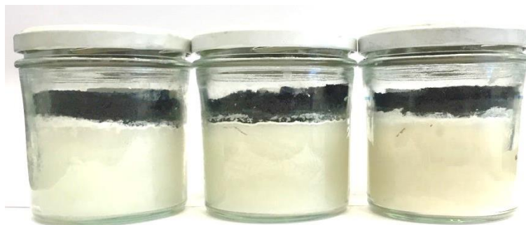
Figure 5. Three samples of SAT with thickening agent with a layer of graphite and SAT on top.
