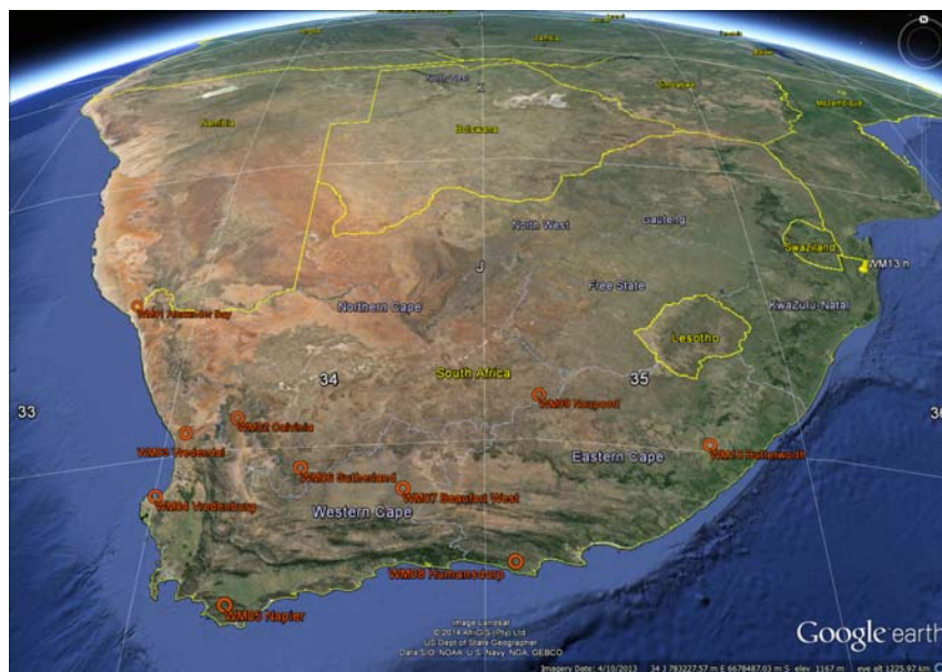
Figure 12. Google Earth image of southern Africa showing the three UTM zones covering the WASA Phase 1 domain: 33, 34 and 35. Each zonal coordinate system is Cartesian and the coordinates can be given in [m] or [km].
