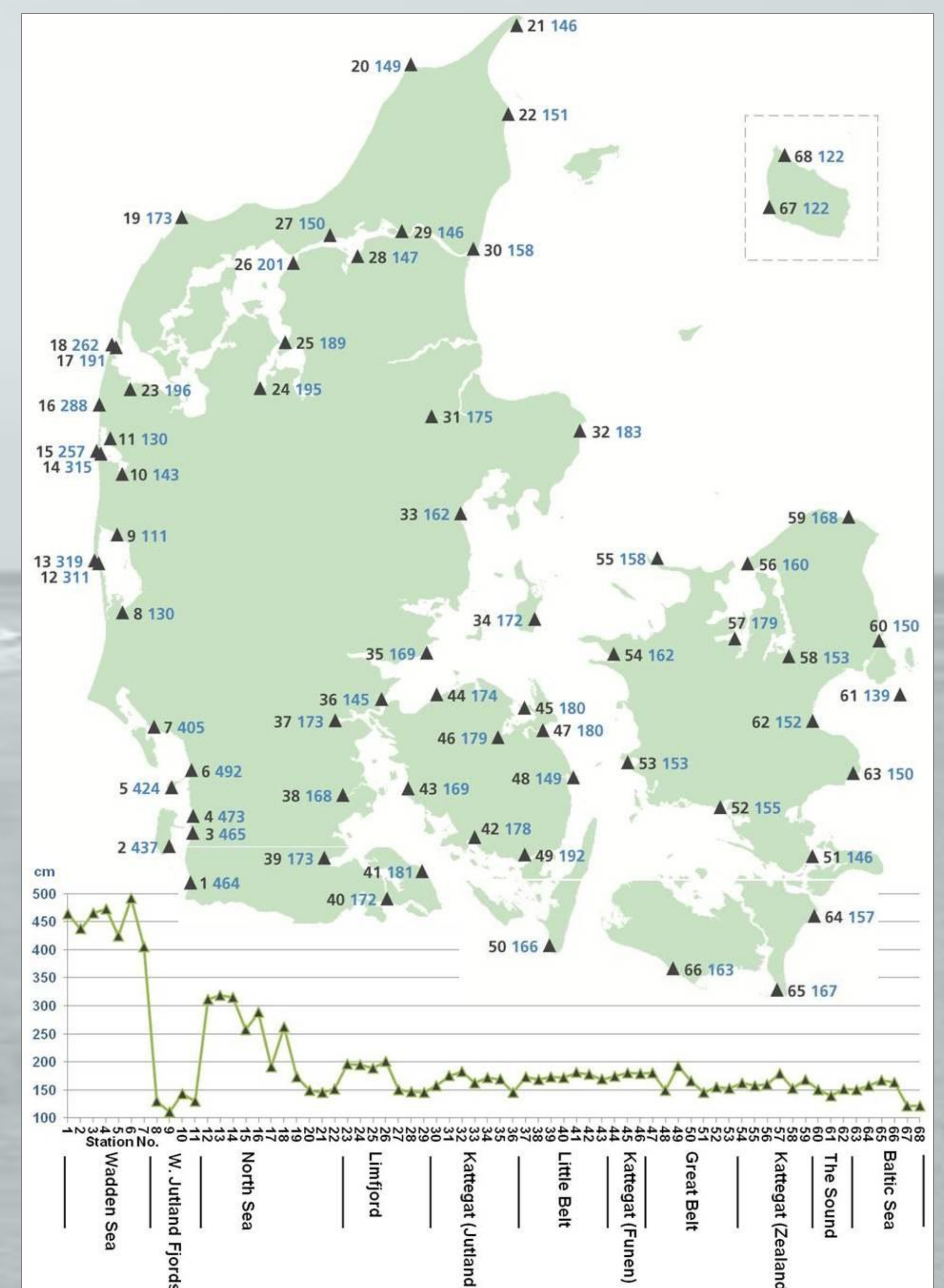
Figure 2 100 y return heights (in blue) in cm above datum (DVR90) for the 68 Danish tide gauge stations according to Sorensen et al (2013). POT from Weibull or Log-Normal distributions. No tides removed
