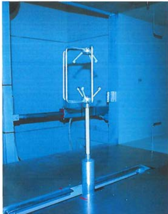
Image 1: Calibration set-up of flow direction test in the wind tunnel of Deutsche WindGuard, Varel. The sensor shown may differ from the calibrated one. Remark: The proportion of the set-up is not true to scale due to imaging geometry.
