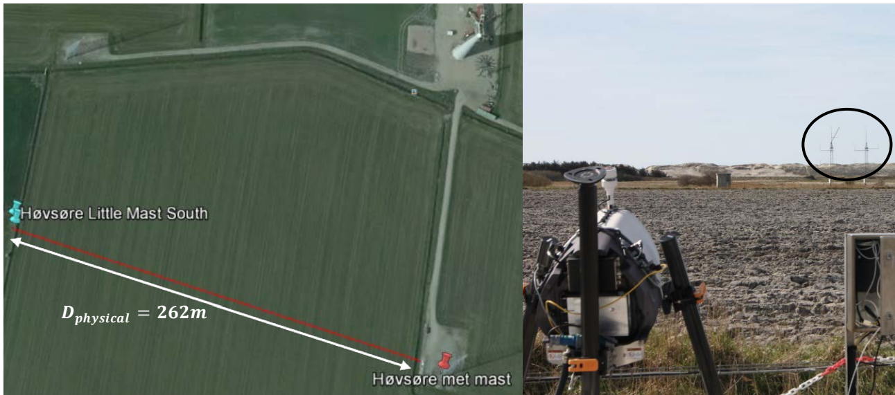
Figure 14. Calibration measurement setup of the ZDM lidar at DTU Wind Energy test site, Høvsøre (DK)
