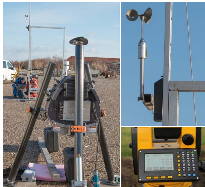
Figure 5. Left: photograph of the measurement setup for ground calibration of the Zephyr Dual-Mode tilt inclinometer. Top right: cup anemometer used as moving hard target. Bottom right: 3D coordinates measurements with a theodolite
