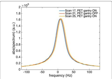
**Fig. 8** Examples of <sup>13</sup>C spectroscopy during PET gantry ON and OFF. Plots show <sup>13</sup>C spectra under conditions of the PET gantry ON and OFF, as denoted in the legend. Spectra are from the voxel with the maximum urea signal and zoomed on the urea peak to highlight the small differences of the spectra
