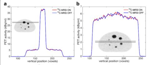
**Fig. 4** PET profiles during <sup>13</sup>C-MRSI ON and OFF. PET line plots of voxels between the *black lines of the inserts*, through **a** the largest sphere (single slice) and **b** background region (10 slices). Conditions of simultaneous <sup>13</sup>C-MRSI ON and OFF are shown as *red* and *blue* colors, respectively
