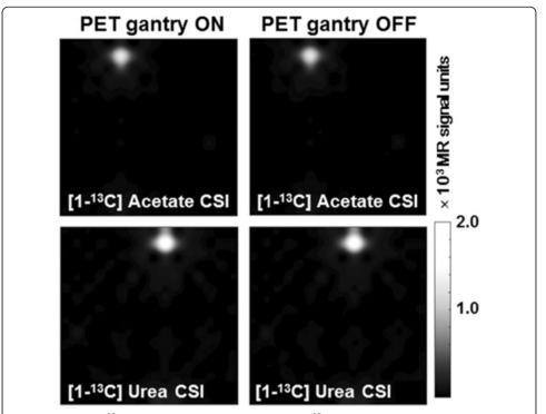
**Fig. 7** Examples of <sup>13</sup>C-MRSI during PET gantry ON and OFF. <sup>13</sup>C-MRSI obtained with the PET gantry OFF (*left column*) and with the PET gantry ON (*right column*). Top row is acetate, bottom row urea metabolite images
