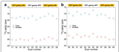
**Fig. 6** <sup>13</sup>C-MRSI SNR for mMR water phantom measurements. Plots show urea (blue *symbols*) and acetate (*red symbols*) SNR for <sup>13</sup>C-MRSI scan numbers 17 to 40. For scan numbers 21–24 and 33–36, the PET gantry was switched off, as indicated by the *yellow bar*. The PET activity was high and low for scan numbers 17–28 (a) and scan numbers 29–40 (b), respectively
