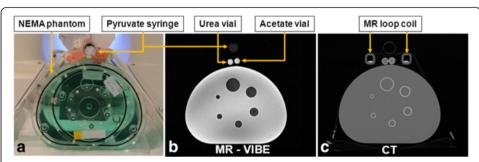
**Fig. 1** NEMA phantom setup. **a** Photo of setup with PET NEMA phantom and pyruvate syringe for hyperpolarized <sup>13</sup>C-MRSI marked with arrows. **b** <sup>1</sup>H-MRI with urea and acetate vials for thermally polarized <sup>13</sup>C-MRSI marked with arrows. **c** CT with cross section of <sup>13</sup>C loop coil marked with arrows
