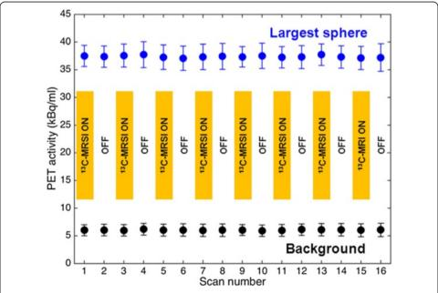
**Fig. 5** PET activity for all NEMA phantom measurements. Measured PET activity in the largest sphere (*blue points*) and in a background region of the phantom (*black points*). *Error bars* are standard deviations on estimates. For odd PET scan numbers, simultaneous <sup>13</sup>C-MRSI was performed, as indicated by the *yellow bars*
