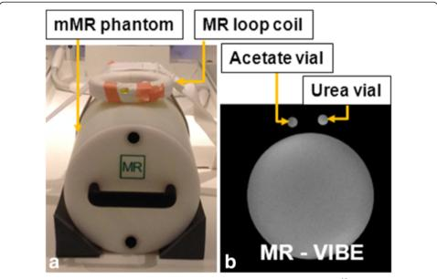
**Fig. 2** mMR water phantom setup. **a** Photo of setup with mMR water phantom. The <sup>13</sup>C loop coil is marked with arrows. **b** <sup>1</sup>H-MRI with urea and acetate vials marked with arrows
