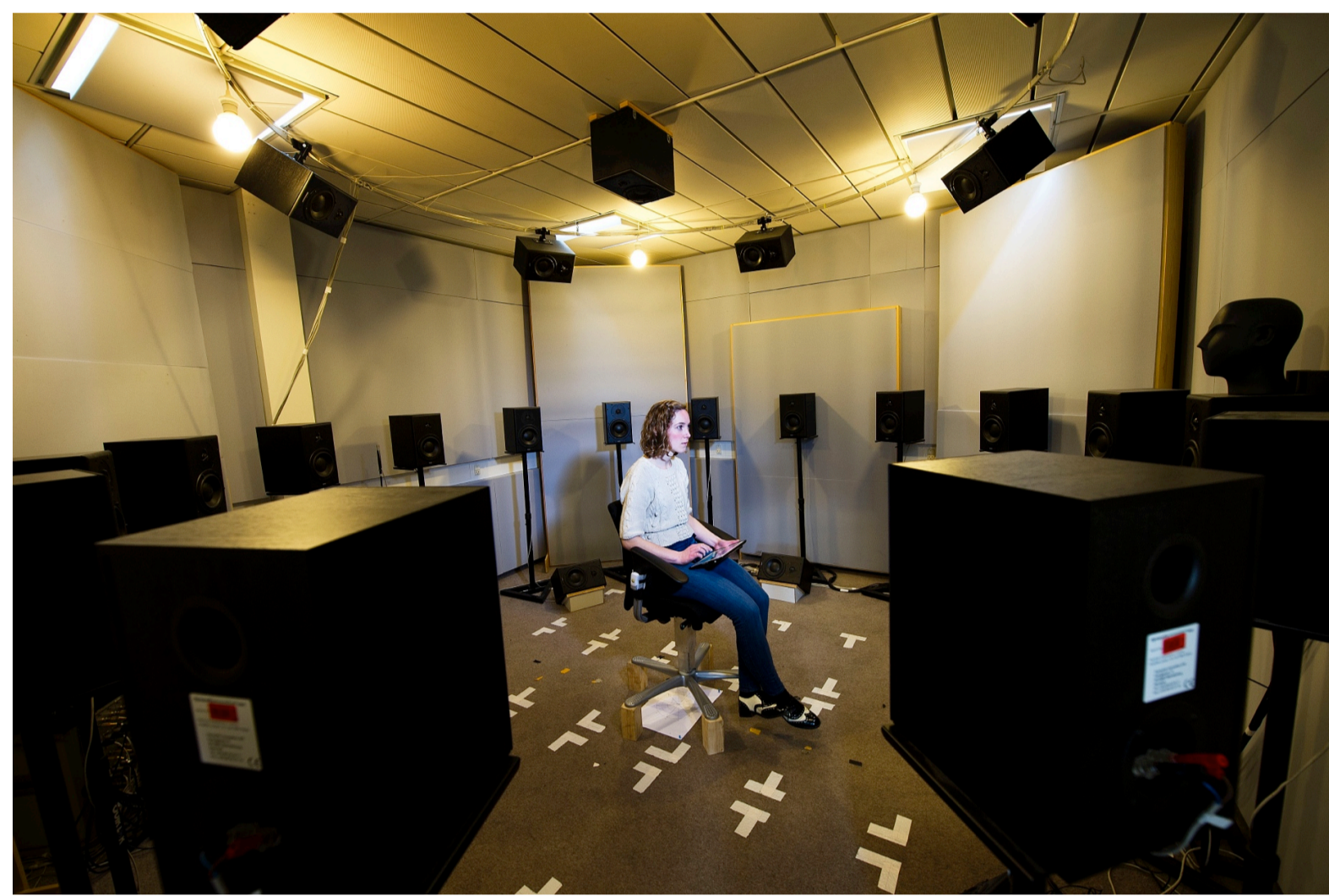
Fig. 1: Photograph of the 'Spacelab' at DTU with a spherical array of loudspeakers for the playback of VSEs.
