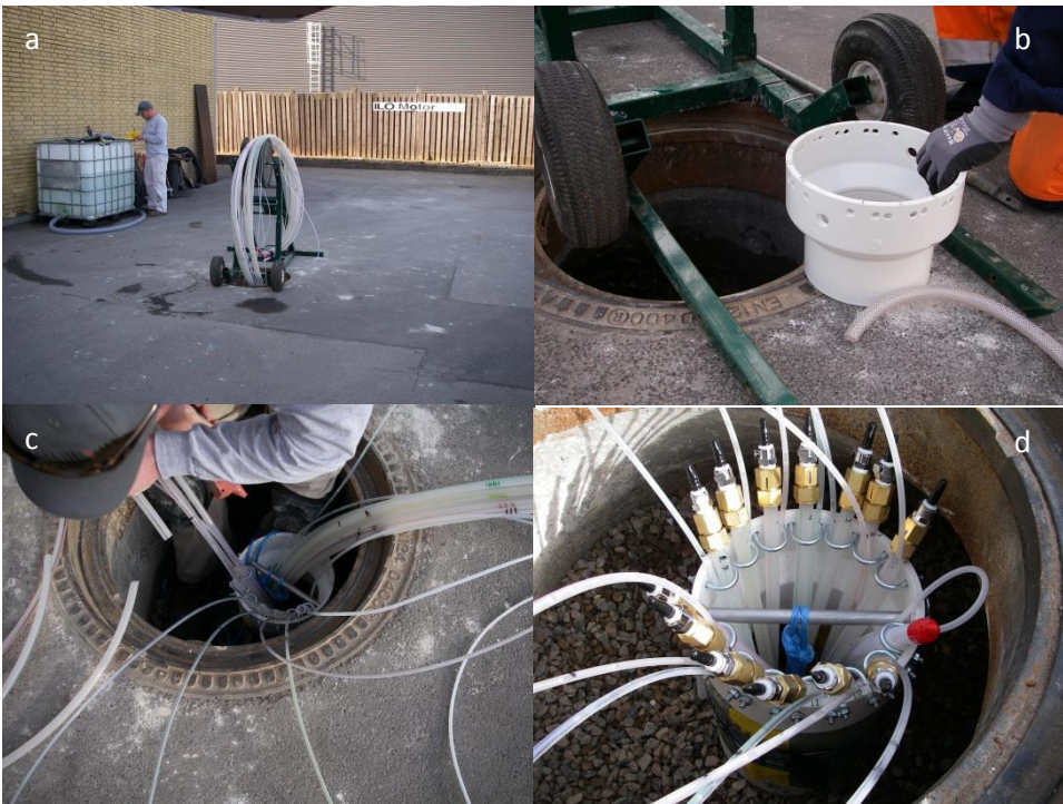
Figure S3: 1) FACT™ on NAPL FLUTE™; 2) FLUTE® transmissivity profiling; 3) Water FLUTE™ a) Inside part of Water FLUTE™ sampling port, b) tubing from the sampling ports held in place in the Water FLUTE™, c) Water FLUTE™ with tapering; 4) Water FLUTE™ preparation
