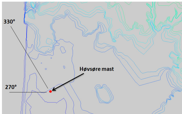
Figure 44: Map of height contours around the Høvsøre test site. Each contour on the map represents a difference in height of 1.8 m.
