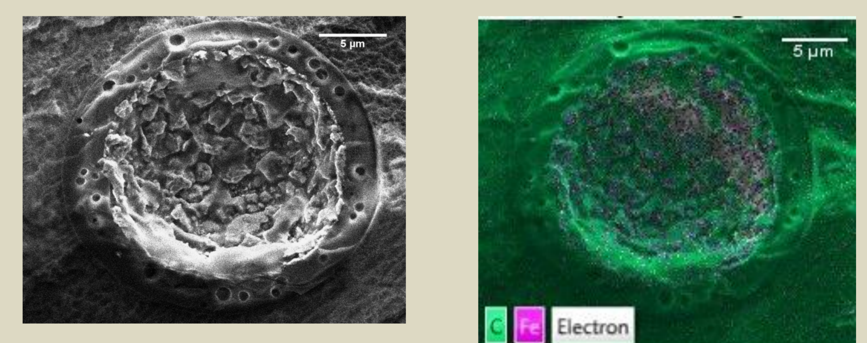
Cryo SEM micrograph showing the cross section of a PMMA microcapsule with encapsulated \text{Fe}_2\text{O}_3 nanoparticles and the corresponding EDS mapping.
