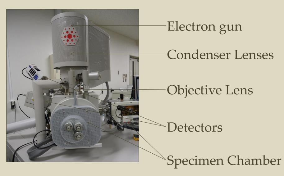
In the high vacuum SEM a finely focused beam of electrons is moved across the specimen one point at the time. The electrons interact with the sample and causes electron emission, which is collected and amplified by an electron detector (Everhart Thornley). The image is assembled –like a mosaic – from the pixels sequentially examined by the beam and displayed on a computer screen.
