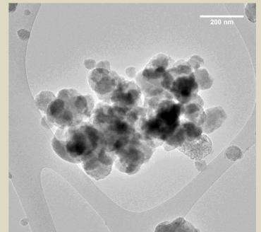
The Black Carbon particles accumulated in Greenland's snow have fewer monomers with a pearl on a thread (chain like) preferential arrangement.
