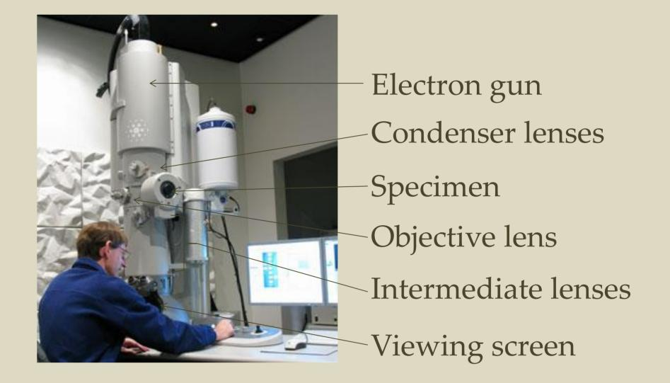
In the bright-field TEM the sample is exposed to a parallel beam of accelerated electrons. The electrons interact with the sample and the transmitted electrons containing structural information are projected onto a vieviwing fluorescent screen. The image is recorded with a CCD camera and displayed on a computer screen.
