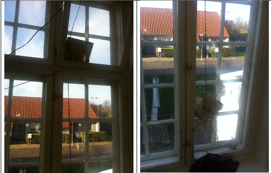
Figure 9 Location of the additional meters in the gap between external and internal frame: on the left is the meter located in the top of the window and on the right the meter is located in the bottom of the window.
