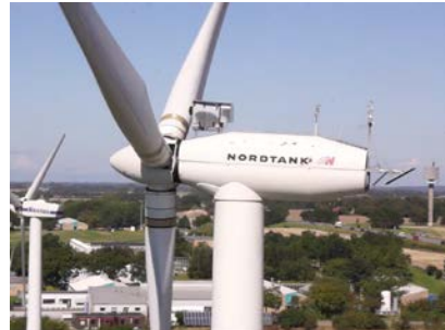
Figure 3 Picture of the DTU SpinnerLidar installed on top of the nacelle behind the rotor (the system was protected from the rain with an aluminium enclosure)
