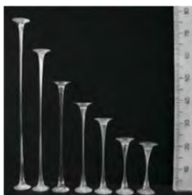
Figure 1: Samples as available after being exposed to different extensional flow rates.
