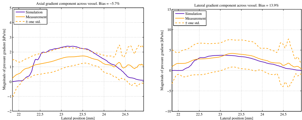
Figure 5: Estimated and simulated pressure gradients along the cross-sectional direction of the constriction. The two graphs show the axial and lateral component of the pressure gradient, respectively.
