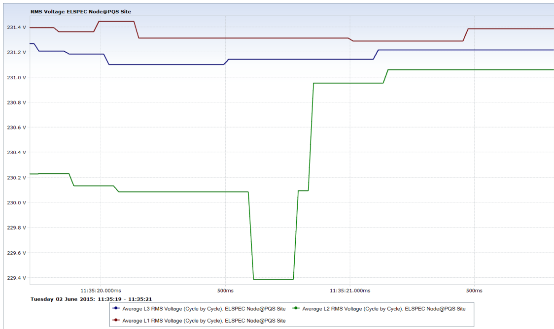
Fig. 24. 11:35 – Event #2: zoom-in of the phase-neutral voltage on phase b
