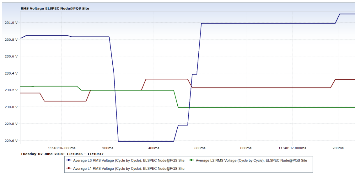
Fig. 26. 11:40 – Event #3: zoom-in of the phase-neutral voltage on phase c
