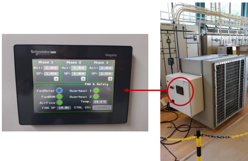
Fig. 4. Phase-independently controllable resistive load and the control interface
