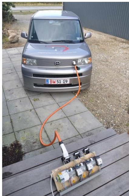
Fig. 5. eBox connected to the ending terminal of the line through a single-phase switchboard
