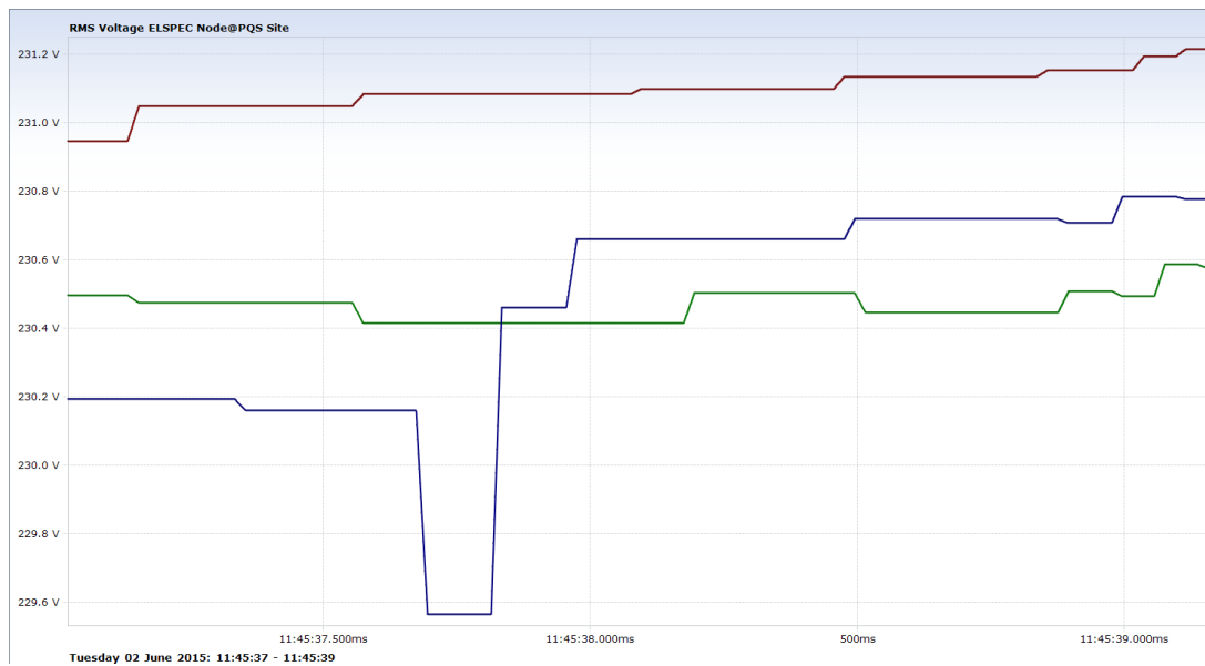
Fig. 29. 11:45 – Event #4: zoom-in of the phase-neutral voltage on phase c
