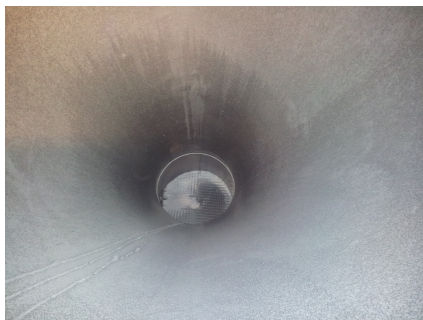
(b) The SFB at the bottom of the dryer chamber.
