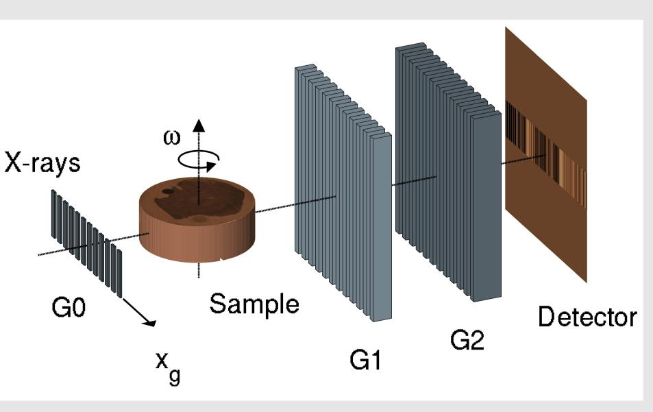
At laboratory-based setups a third grating, G0, is included to assure satisfactory coherence in the x-direction. A rotation sample stage can be included for tomography.
