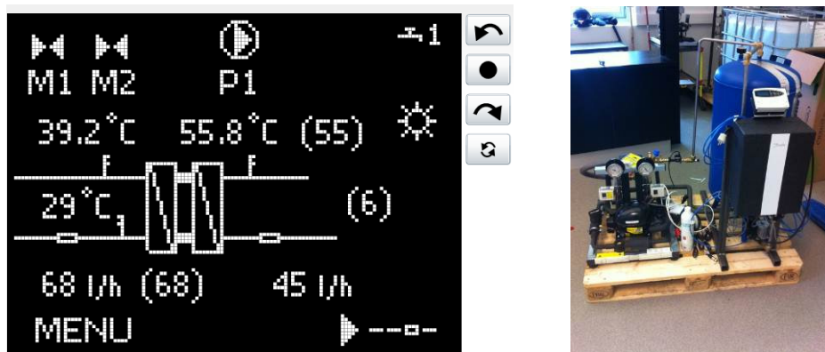
Figure 9: Left: Display of electronic controller, accessed via web portal (ECL portal). Right: System test equipment
