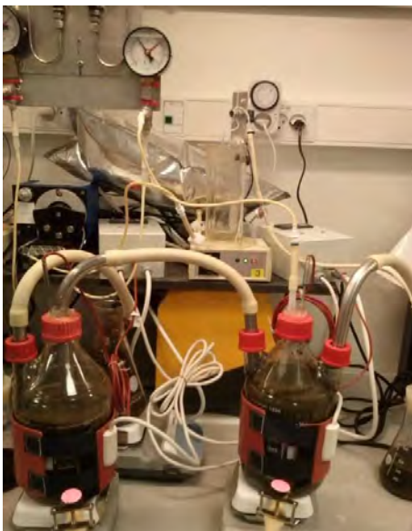
Fig 1: Two-stage reactor configuration.
