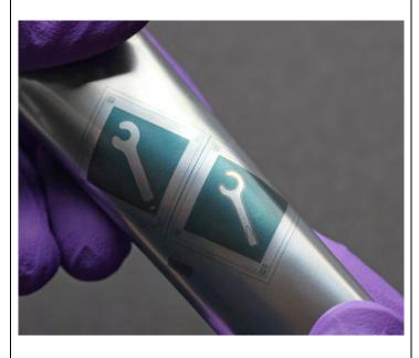
Flexible plastic foil with embedded plasmonic color meta-surface decoration. The color appears from a thin film of aluminium deposited on top of a nanotextured surface.
