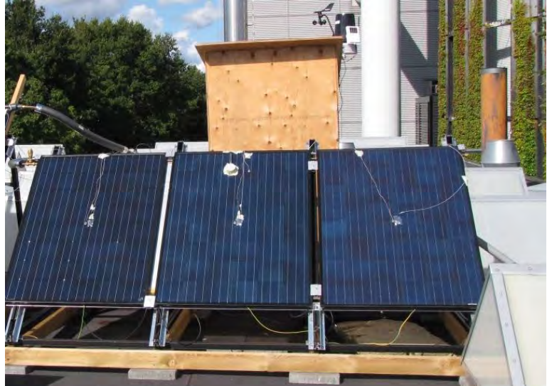
Figures. Experimental chamber with PCM radiant ceiling (left) and PV/T panels (right).
