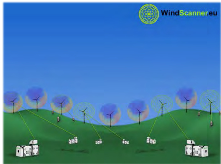
Inflow and wakes around turbines exposed to wind and turbulence in complex terrain are scanned in 3D space and time from WindScanners.
